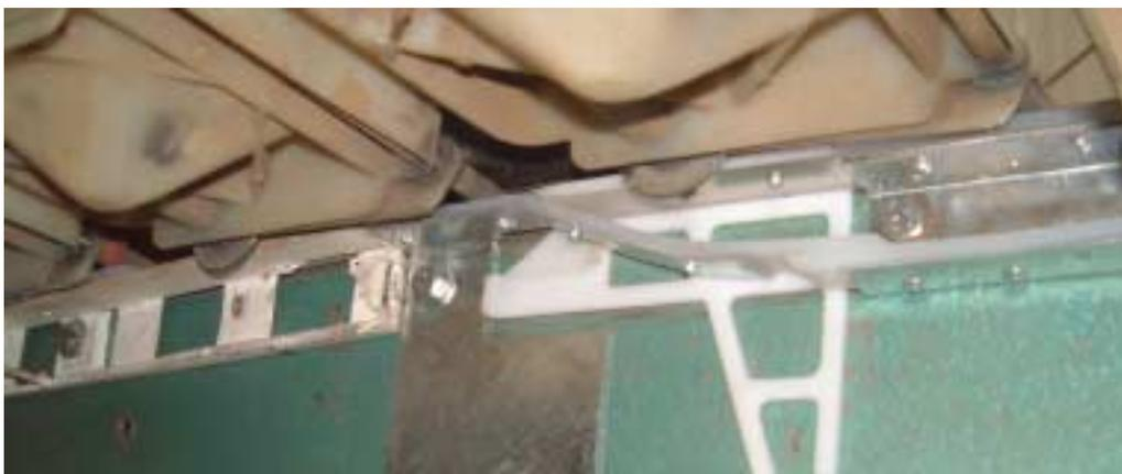
**The new solenoid gate installed on a 6 Lane MacDonalds sizer in the USA.**
