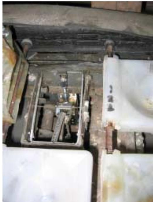
**Figure 3. Activating the scale arms with solenoids**
