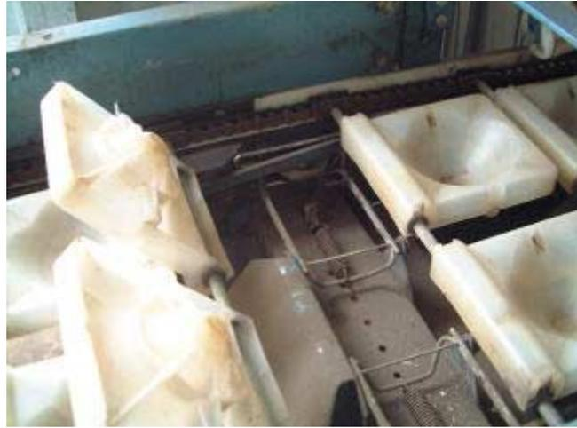
**Figure 1 . A typical mechanical sizer**
