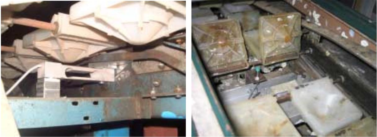
**Figure 2. Loadcell installation examples on Treeways and FMC mechanical sizers.**
