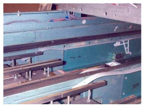
way. The magnets are removed and replaced using a Treeway's type gate system and utilising 24 volt DC solenoids with new pressings. The advantage of this system is that the gates are always shut. Therefore the cups stay up all the way to the end of the machine unless the control system opens the gate to allow for the fruit to drop, reducing the number of problem areas from say ten to one.
